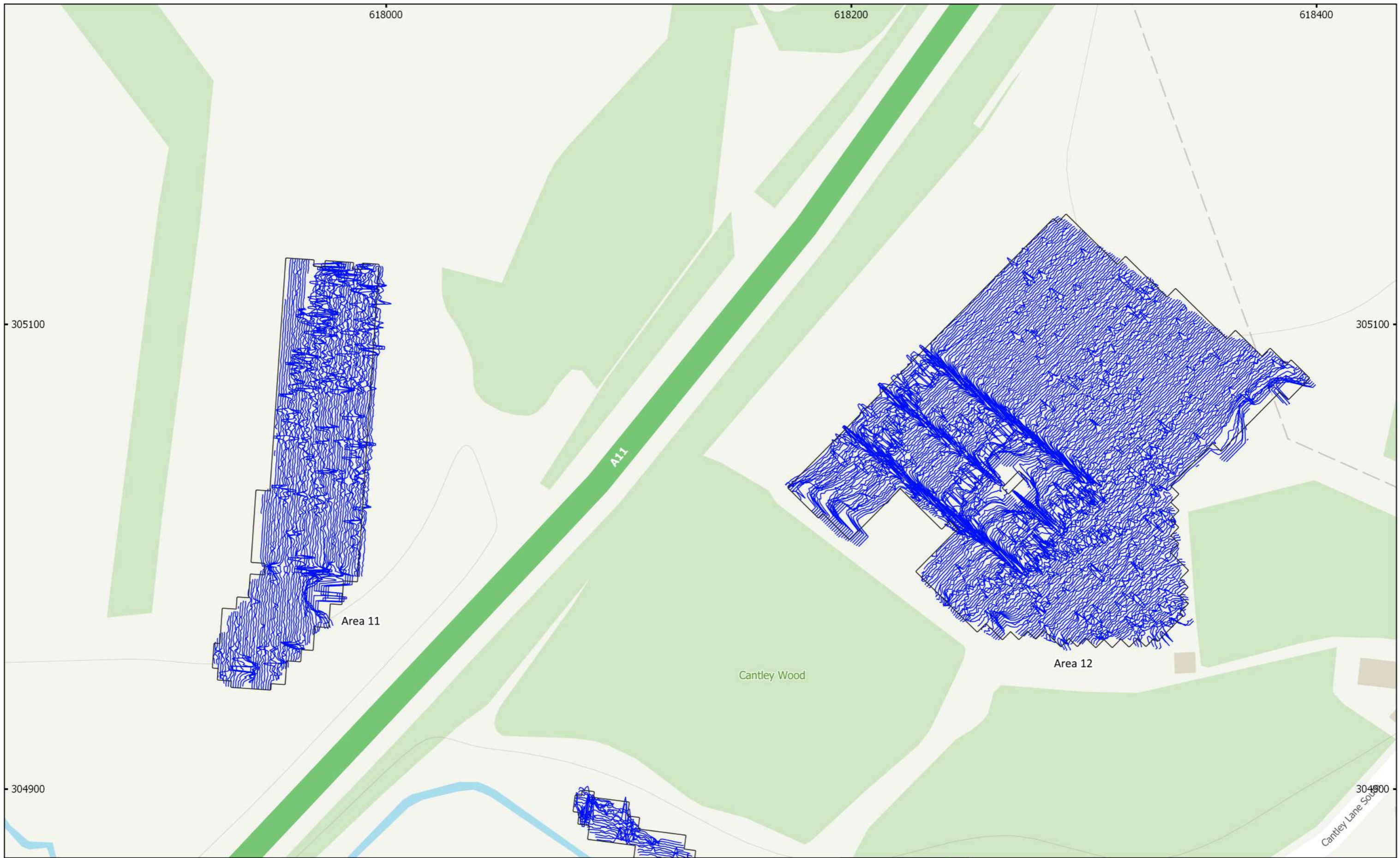
MSTG812 - A47-A11 Thickthorn Junction, Hethersett, Norfolk Figure 15 - XY Trace Plot (Areas 11 & 12) 30nT/cm at 1:1,500 @ A3 Copyright Magnitude Surveys Ltd 2020 Contains Ordnance Survey data © Crown Copyright and database right 2020
